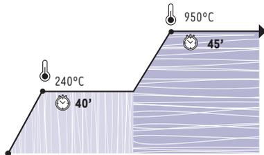
If the indicated drying times and pre-heating temperatures are not observed, slight fissures in the muffle surface may occur; they are of no importance for the cast object.
