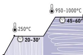
If the indicated drying times and pre-heating temperatures are not observed, slight fissures in the muffle surface may occur; although this will not affect the casted piece.
