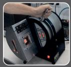
A quarter turn is sufficient to complete the casting in the cylinder. You can monitor the process thanks to the screen.
