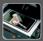
...and insert it into the fusing unit. Closure. Press START again to start the vacuum. After a short period of time the material will be melted.
