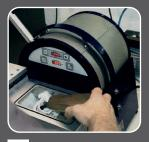
Insert the crucible with the material into the quartz glass tube inside the inductor.
